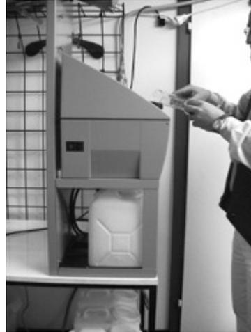
The processor should be positioned with the feet in location holes in the reclamation unit. The drain outlets for the three chemistry baths connect with the storage containers without the need of interconnecting hoses. Drain hoses for rinse water and the water jacket must be connected. When lowering the processor, take care that the outlets of the processor align to the tubes of the reclamation rack.
