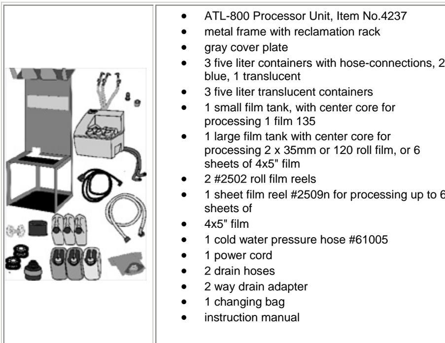
The ATL processor should be positioned on a firm, dry and level surface, close to a cold water supply, drain and power source. The water supply should be capable of supplying cold water at a pressure between 2 and 6 bar (36 to 108 p.s.i.). If the water pressure is higher than this, a pressure reducer should be used. The AutoLab should be installed in accordance with local water and sewerage regulations.
