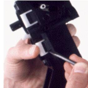
9.0 Insert the white retention clips. Make sure the bottom edge of the clips is underneath the black ledge molding located on the rear side of the lift arm. Use a small standard blade screwdriver to "encourage" the clip over the ledge molding.
