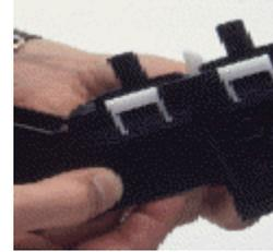
8.0 Release the white retention clips by pressing inward at the base of each clip leg.
