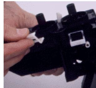
10.0 Press or push the coupler back into its original position.
