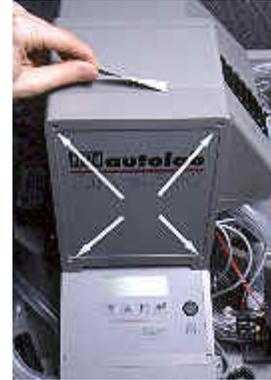
9. Remove the front cover of the electronics head.
