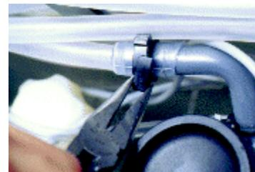
5) Disconnect the first four (4) air lines from the bottles, keeping the black plastic 90° angle elbows attached to the hoses.
