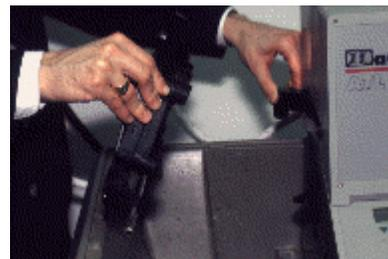
4) If you have a floor standing processor (model 4170, 4270, 4171, or 4271) and are reclaiming chemistry in the 15 liter bottles, remove each hose in the sink area by pulling or lifting it off of its receptacle. Hold the chemical drain arm toward the rear of the processor and at the same time, remove the reclamation unit by sliding it or lifting it upward off of its mounting bracket.
