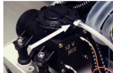
4) Located on the left side of the lower motor unit you will observe a bracket that wraps around the power cord and grips the motor unit. Pull the bracket away from the motor unit using your standard blade screwdriver to assist. Then lift the upper head upward and toward the right. Rest it in the trough.
