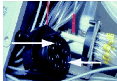
**DO NOT** remove the air hoses from the left half of the front/back bottle (air) switch!
