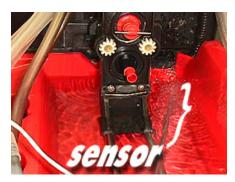
Operational Point: The water bath temperature sensor is located inside of the pump housing (the channel that draws water up into the upper water bath). Therefore the reason you are placing the chemical temperature sensor into the "waterfall", is because the "waterfall" is as close to the water bath temperature sensor as you can be.
