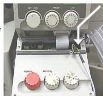
2.6 Follow the wires up from both the CHE and WA black connectors until you locate the small black tube-like piece with a nylon cap fitted into the end of the tube. The two wires connected to each tube attach directly to the black connectors CHE and WA.
