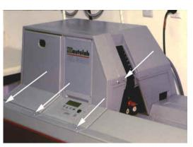
2.2 For ATL-2+ ONLY: Remove the front bottle cover as well as the 3mm cap head screw and washer located near the left cover hinge.
